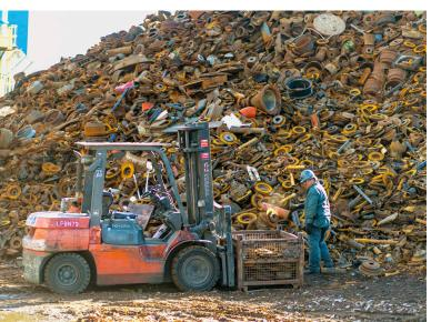
AB&I uses tons of post-consumer scrap metal annually to produce cast iron soil pipe and fittings which further reduces the impact on our landfills.
