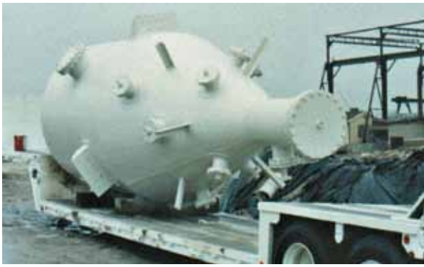
VERTICAL TORICONICAL TANK Custom, 108" cone.
